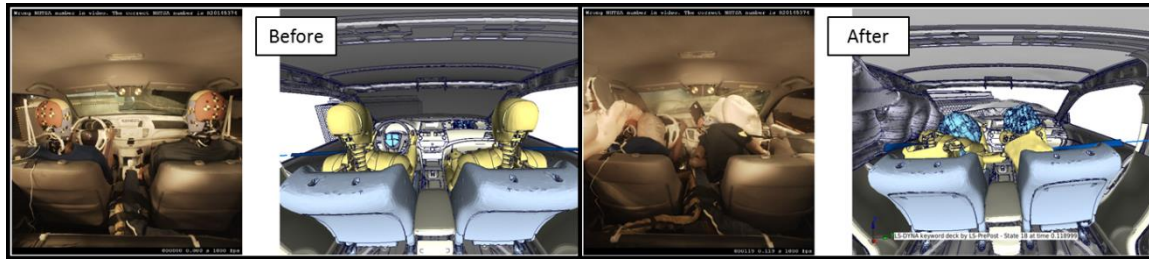
Figure 2. Test vs CAE simulations using THOR dummy models at 0ms (before crash) and 120ms (after crash).
